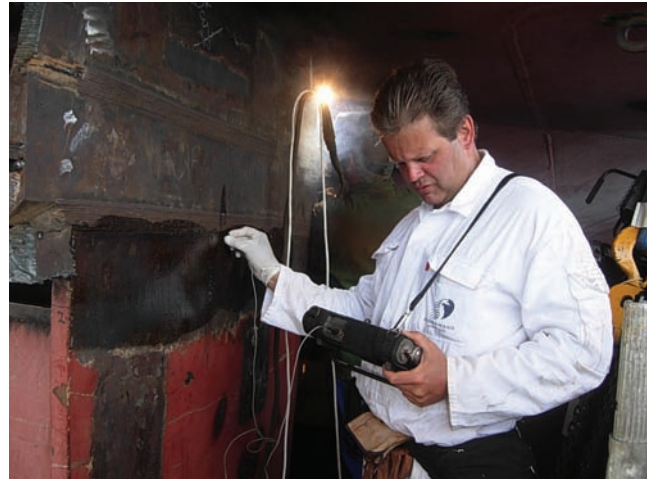
Fig. 11 — Inspector Mark Thury performing an ultrasonic inspection of a complete-joint-penetration weld.
