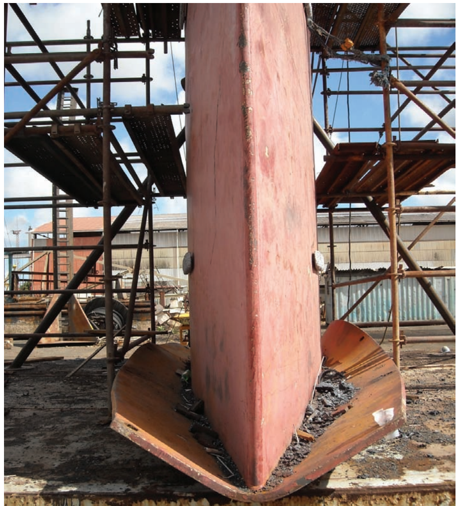
Fig. 5 — The bent rudder bottom plate.
